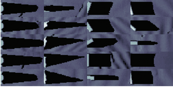
FIGURE 14: Snapshot of the shadow of the four targets (from left to right: Manta, Rockan, Cube and Cylinder) to classify with different orientations and backgrounds. The pixel size is these target images is 5 cm. The size of each snapshot is 1.25 \text{ m} \times 2.75 \text{ m} .
